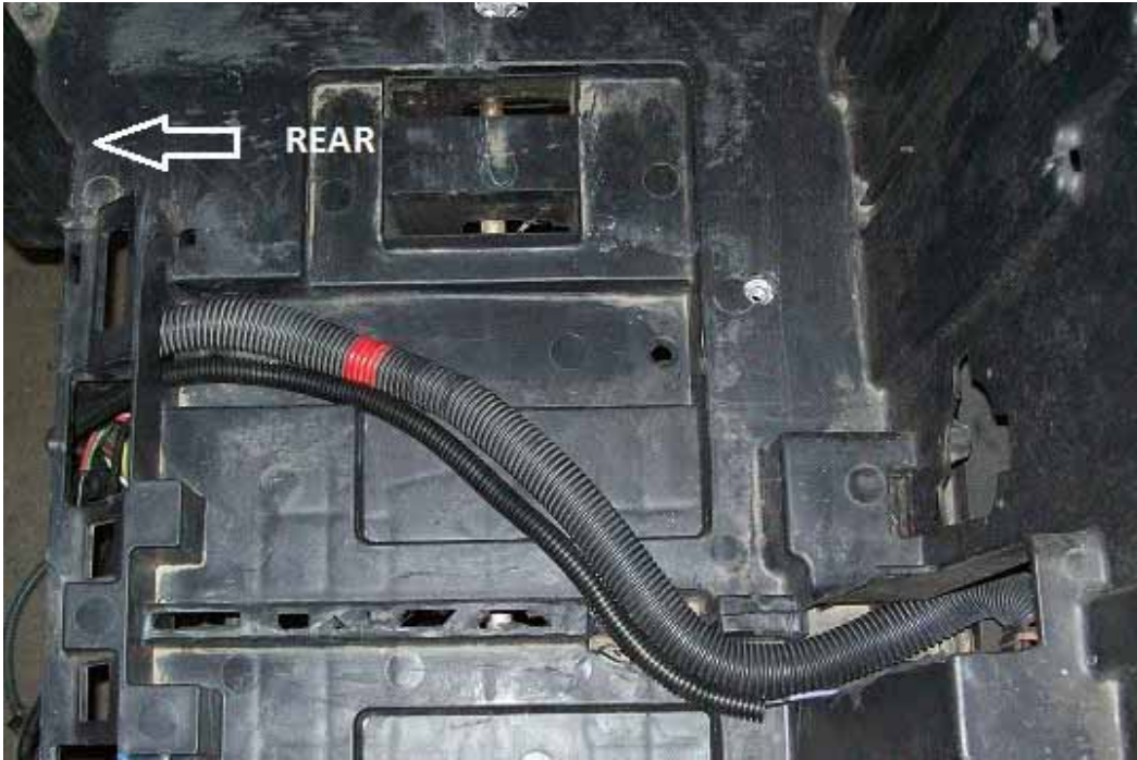
Fig. 10- OEM wiring harness routing
